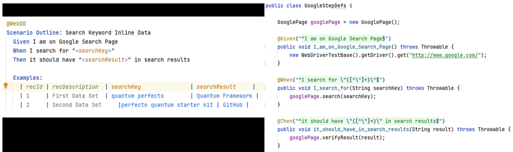
Figure 9.6 – A Cucumber test scenario in Gherkin with a Selenium-based step definition methods
