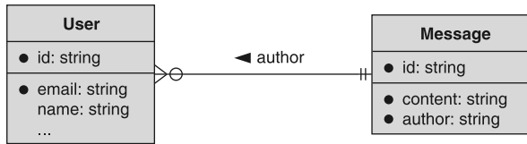
Figure 4.3 A message resource contains a reference to a specific user who authored the message.
