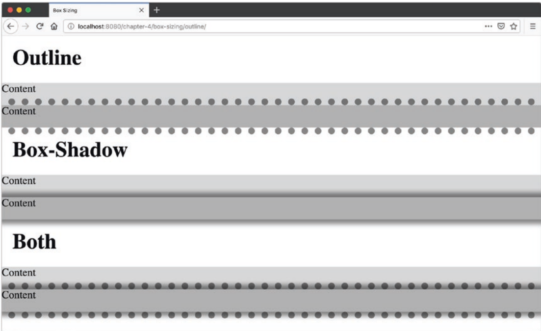
Figure 4-9. Box-Shadow and Outline Do Not Occupy Space in the Layout
