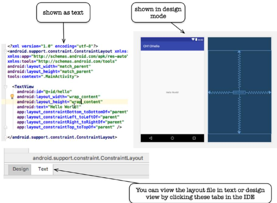
**Figure 3-4.** Design mode and text mode editing of layout files
