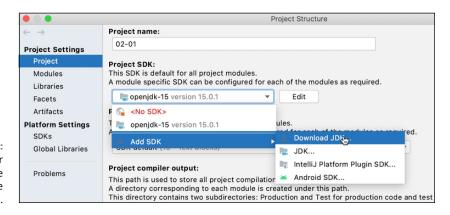
FIGURE 2-12: Finding your way around the Project Structure dialog box. After selecting Project, look in the dialog box's main body for a Project SDK dropdown list. In the drop-down list, choose Add SDK → Download JDK, or select a JDK that's already in the list.
