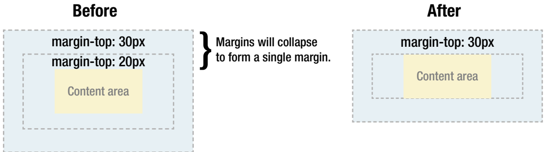
Figure 3-8. Example of an element's top margin collapsing with the top margin of its parent element
