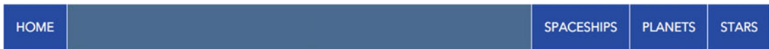
Figure 6-30. Using margin-right: auto on the first item eats up all the space that’s left, pushing the rest of the items to the right
