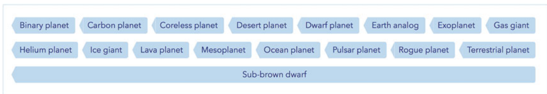
Figure 6-51. The last tag becomes very wide when wrapping onto the last row by itself and growing to fill the space
