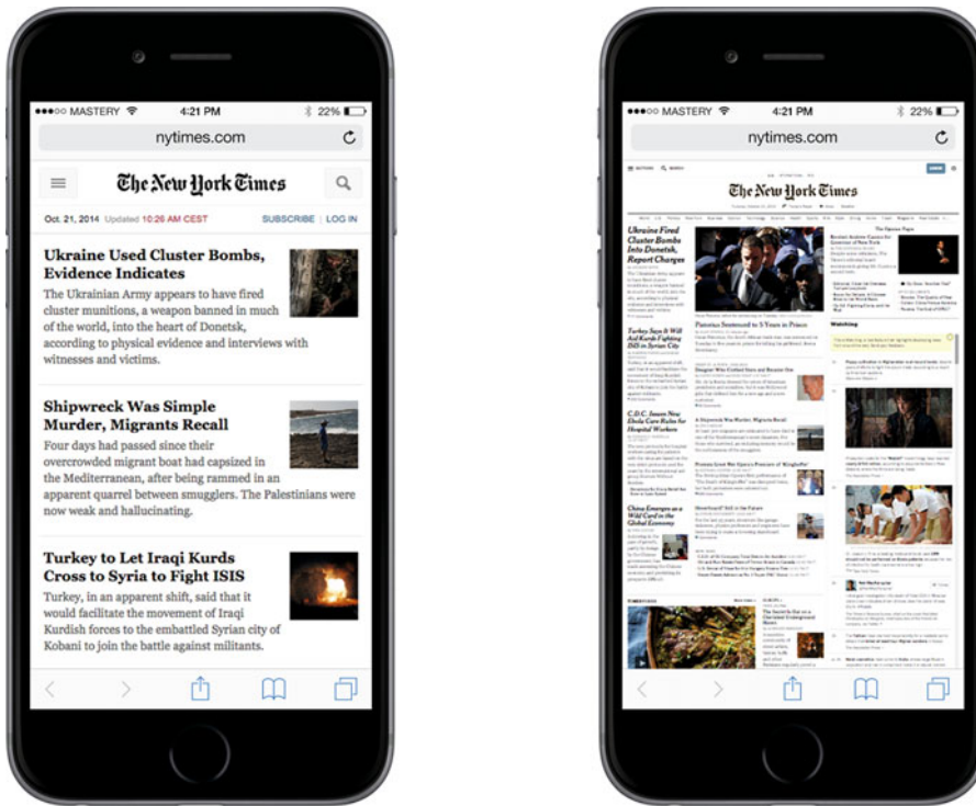
Figure 8-8. The mobile site for the New York Times website uses the ideal viewport for layout (left). If you switch to the “Desktop” site, you get the zoomed-out default viewport look (right), emulating a 980-pixel width.
