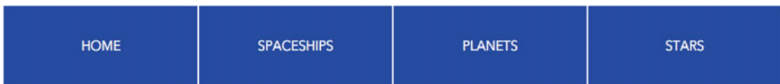
Figure 6-22. Adding a height and vertical centering to list items displaying as table cells
