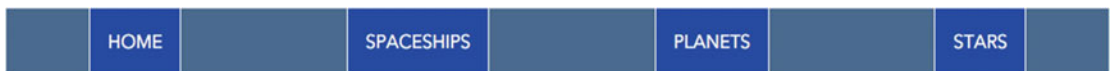
Figure 6-29. Using justify-content: space-around. Space is divided equally and placed on both sides of each item. Note that space between items does not collapse
