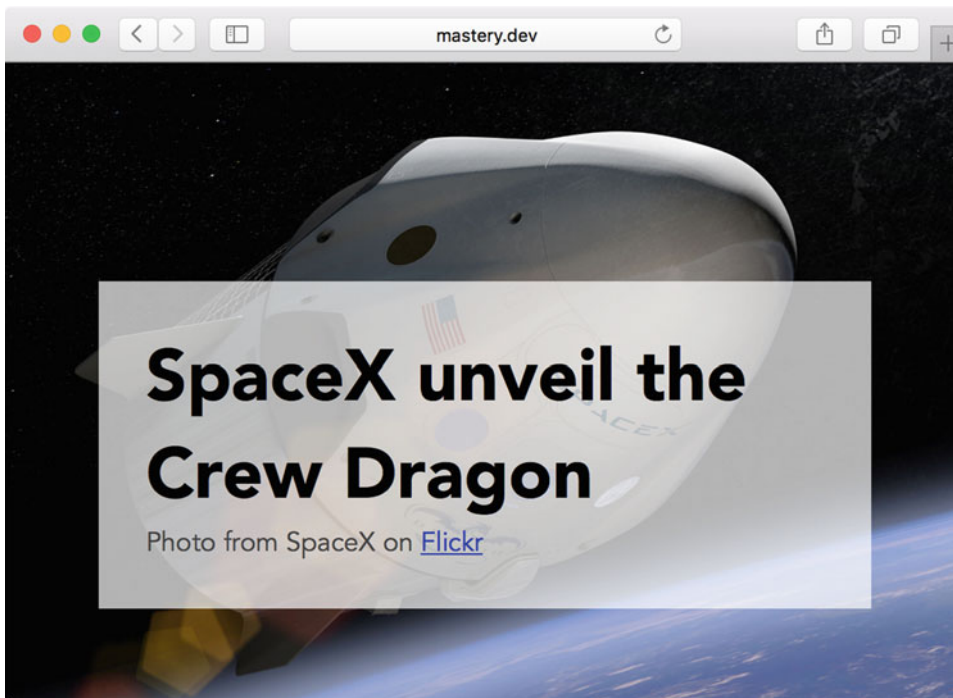
Figure 6-6. At a smaller screen size, the text will wrap as the box grows upward
