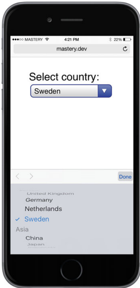
Figure 9-29. A select element on iOS doesn't display the options underneath the select at all, but triggers a rotator-type widget at the bottom of the screen instead
