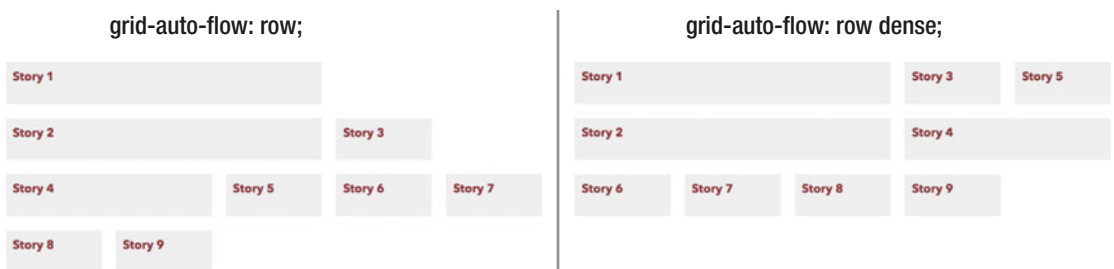
Figure 7-26. When items span several cells, the default sparse algorithm can cause gaps. When using the dense algorithm, the items are more efficiently packed
