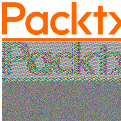
Figure 4.1 – Encrypting an image (the Packt logo at the top) with AES-ECB (middle) and other AES modes (bottom)
