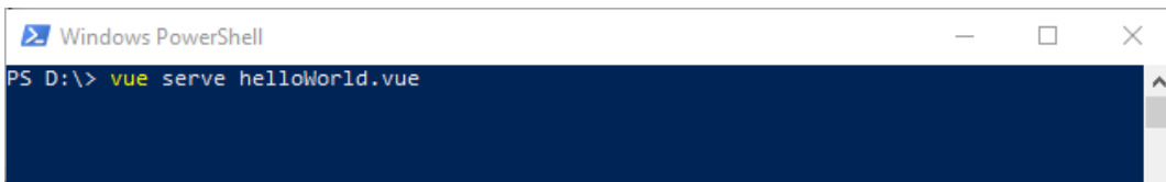
Figure 3.6: The vue serve command is running on a file in the D:\ directory
