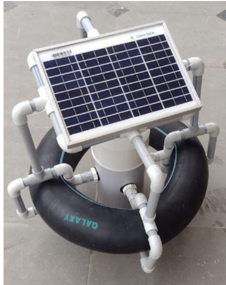
Figure 10-3. Data buoy designed for monitoring water-quality parameters
