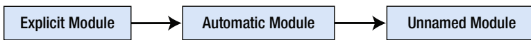
Figure 4-15. An automatic module acting as a bridge between an explicit module and an unnamed module
