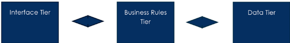
Figure 2-5. Three-tier modular application design
