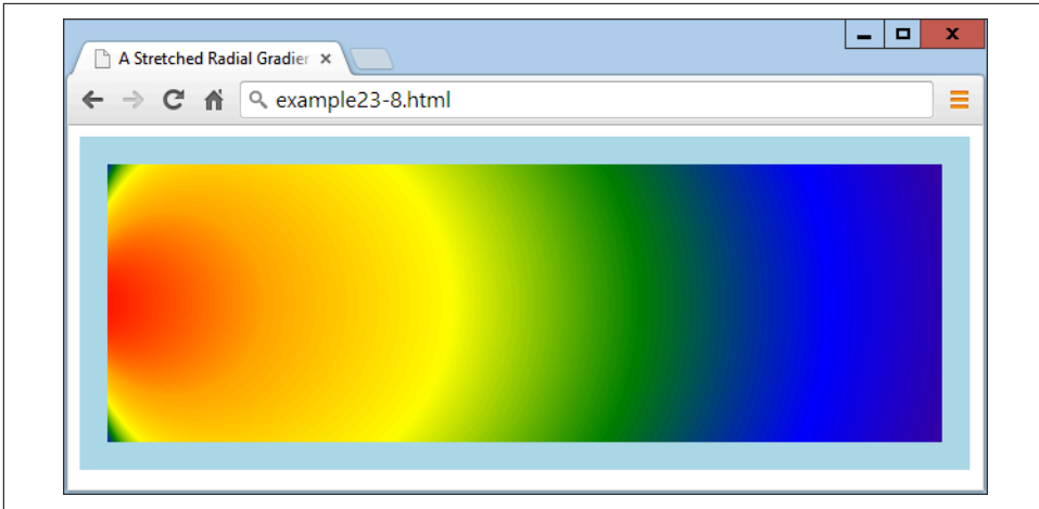
Figure 23-7. A stretched radial gradient
