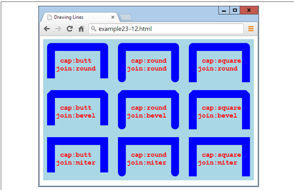
Figure 23-11. All the combinations of line caps and joins
