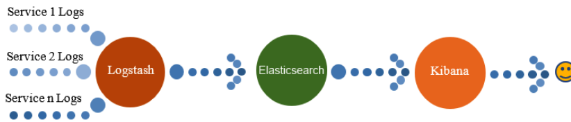
Figure 12.1 – Log flows in the ELK stack
