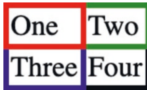
Figure 4-7. Borders are now collapsed
