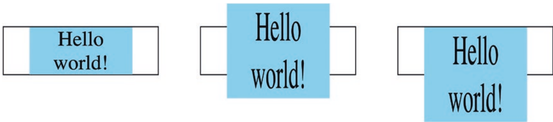
Figure 8-11. No scale (left), scale with origin at center (middle), and scale with origin at top (right)
