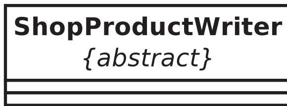
Figure 6-3. An abstract class defined using a constraint
