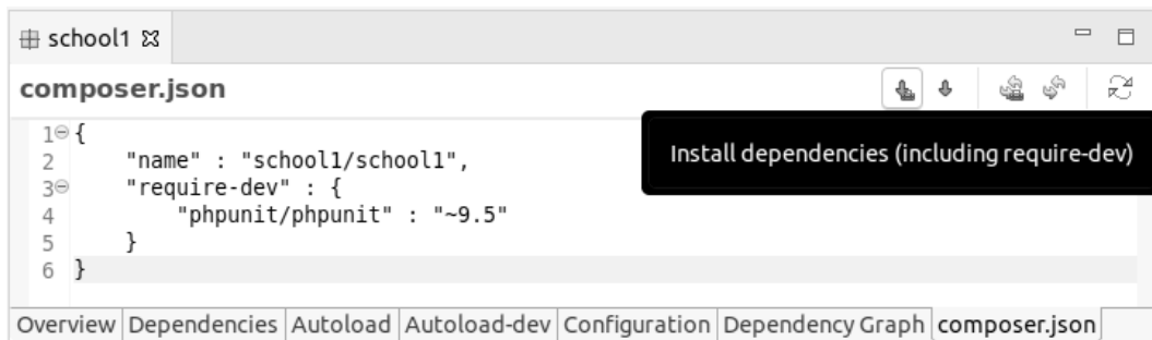
Figure 3.12 – Installing dependencies with Composer
