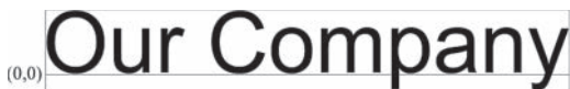
Figure 21.6 Coordinates of the bounding box are given relative to the baseline. The origin of the coordinates is shown here as (0, 0)
