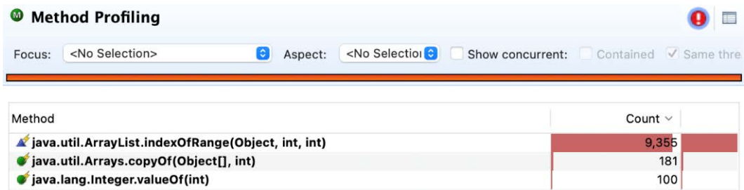
Figure 7.3 – The computation time is limited by busy method execution
