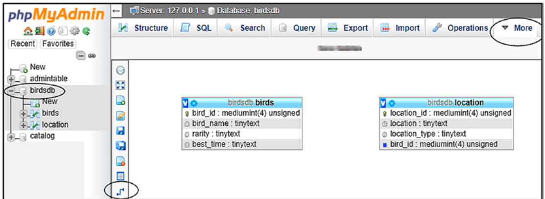
Figure 9-5. Positioning the tables ready for joining
