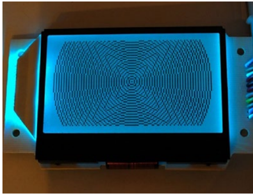
Figure 8-1. Monochrome LCD Credit: Adafruit, adafruit.com
