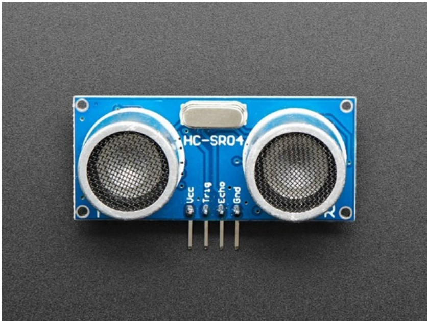
Figure 10-4. HC-SR04 Ultrasonic Sensor Credit: Adafruit, adafruit.com
