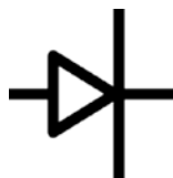
Figure 2-22. The Diode Schematic Symbol
