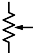
Figure 6-4. The Potentiometer Schematic Symbol
