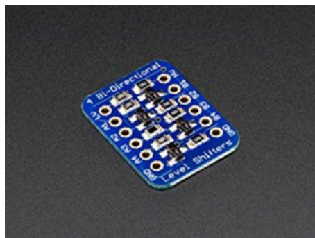
Figure 2-38. Logic Level Converter
