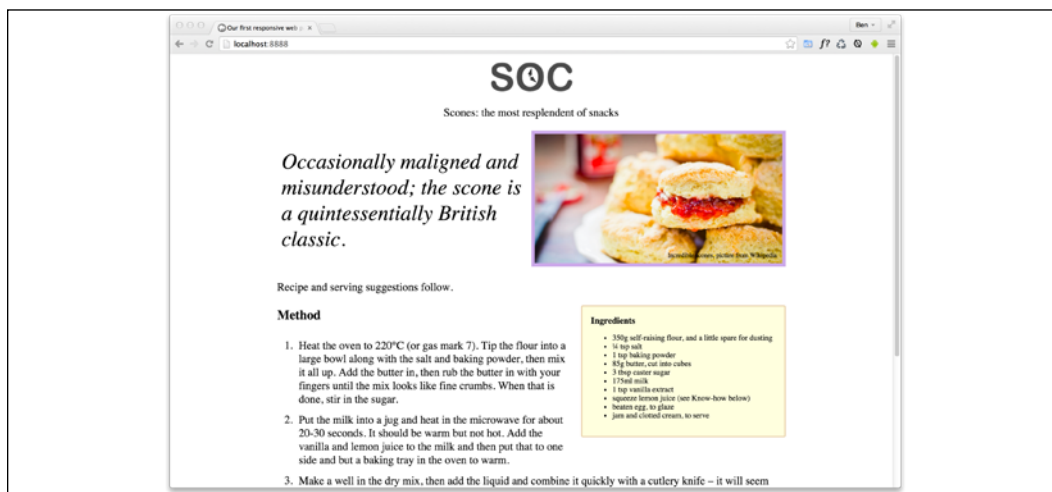
Figure 1.7: With a few rules added within a media query we get a different layout for larger screens
