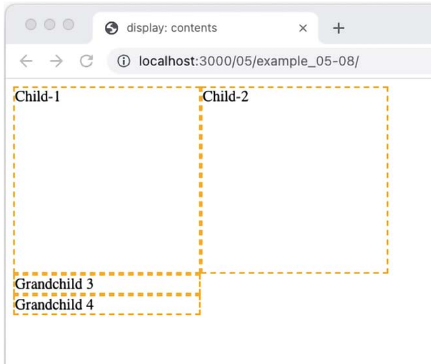
Figure 5.17: By default, descendants of grid items cannot take part in the grid
