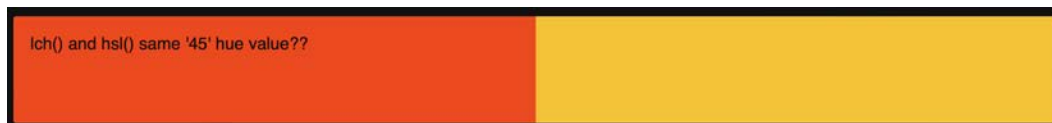
Figure 7.5: Setting lch and hsl to what you think should be the same color does not produce the same color!
