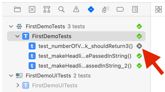
Figure 3.7 – Click the diamond next to the test in the test navigator to run this test
