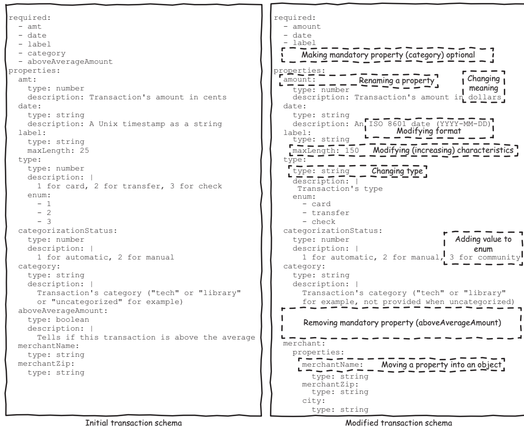
Figure 9.2 How to introduce breaking changes in the list transactions goal's output
