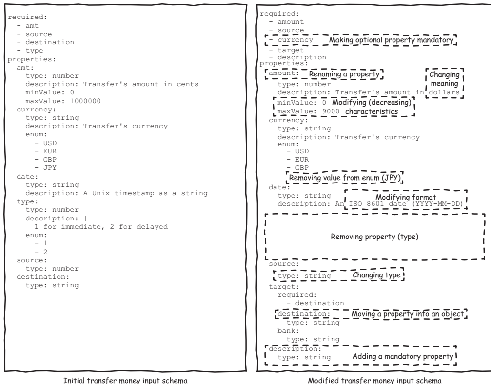
Figure 9.4 How to introduce breaking changes in the transfer money goal's input data
