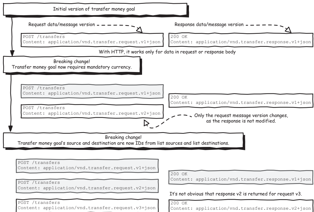
Figure 9.14 Data (or message) versioning with content negotiation
