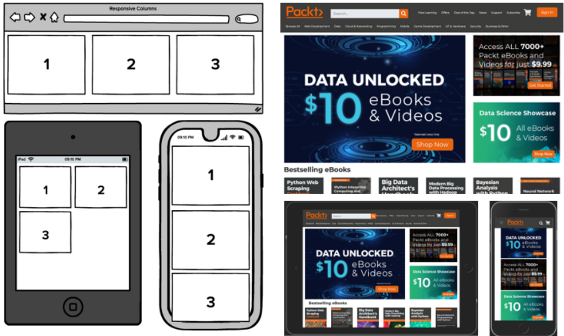
Figure 6.2: A wireframe of a responsive website stacking content, and an example of stacking in practice with the Packt website
