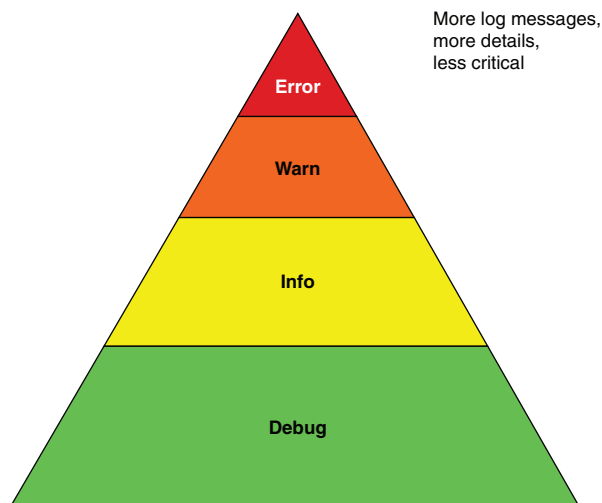
Figure 5.10 The log severity pyramid. On the top are the critical log messages that usually require immediate attention. The bottom represents the log messages that provide details you’ll rarely need. From the top to the bottom, the log messages become less essential but greater in number. Usually, the debug-level messages are disabled by default, and the developer can choose to enable them if their investigation requires fine-grained details about the app’s execution.
