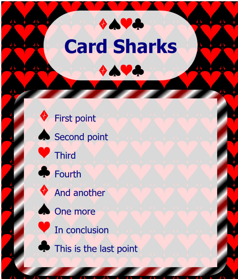
Figure 3-2. A web page using SVG graphics as CSS backgrounds, bullets, and borders
