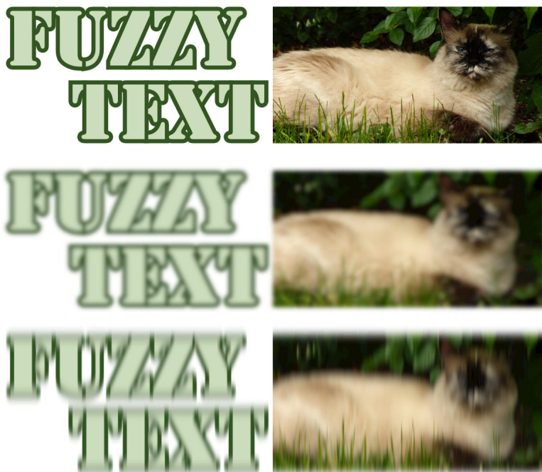
Figure 16-1. Blur filters applied to SVG text and an embedded photo: (top) unfiltered, (middle) bidirectional Gaussian blur, (bottom) vertical motion blur
