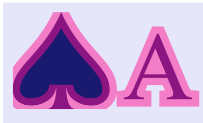
Figure 13-3. Strokes extending beyond the edge of a symbol with (default) hidden overflow
