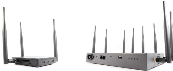
Figure 11.10 – Using a Wi-Fi Pineapple as a jammer
