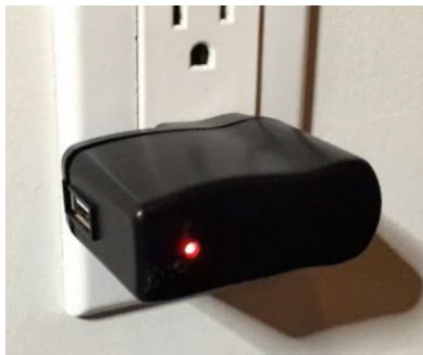
Figure 7.7 – A keylogger hidden inside a USB charger
