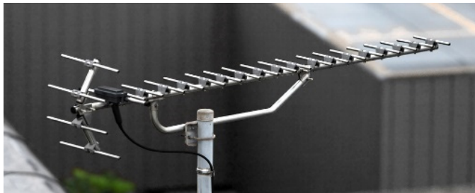
Figure 11.9 – Yagi antenna (by Tennen-Gas – own work, CC BY-SA 3.0)
