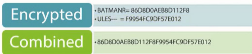
Figure 7.5 – How LM hashes are created
