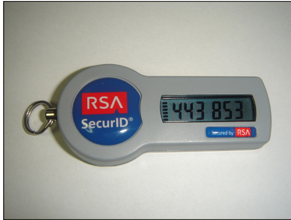
FIGURE 5-4: An RSA SecureID brand one-time password generator hardware token.
