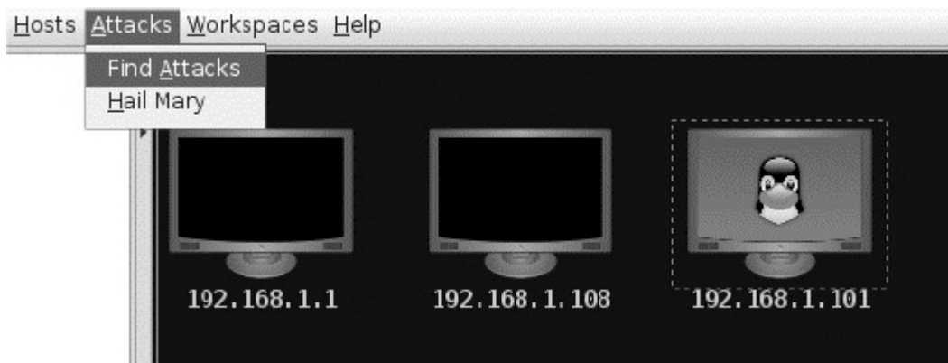
Figure 11-8: Using Armitage to quickly scan all addresses
