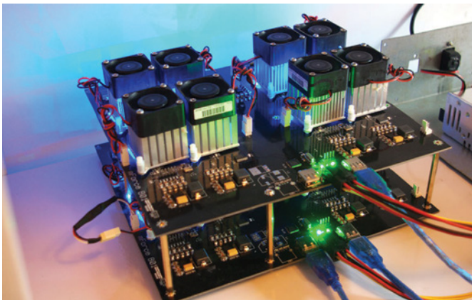
Figure 14.2: FPGA used for cracking hashes
