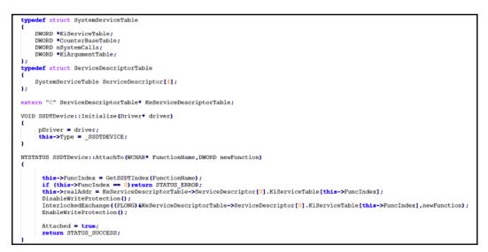
Figure 7.8 – The SSDT hooking code from the winSRDF project
