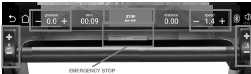
Figure 15-27: Software and physical buttons that allow a user to stop the treadmill
