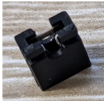
Figure 7-12: A jumper pin, also known as a jumper shunt or shunt
