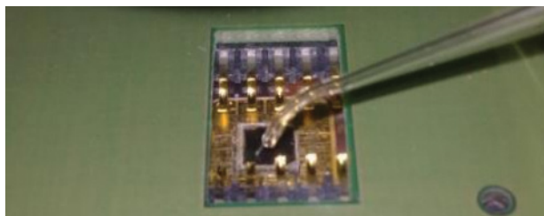
Figure 5-28: Optical fiber laser fault injection (source: Riscure)
