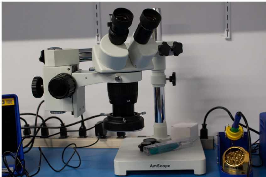
Figure A-11: A low-cost AmScope single-boom optical microscope, with a total magnification of 10x or 20x (switchable)
