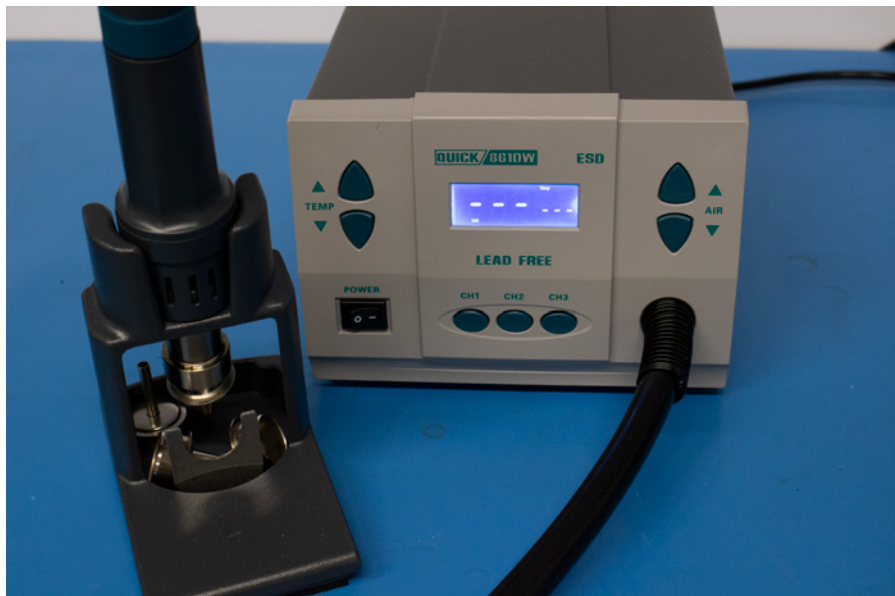
Figure A-6: The Quick 861DW is a good mid-range hot air gun.
