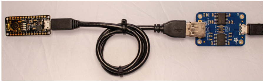
Figure 6-3: An isolator from Adafruit (PCB on the right) and our target (PCB on the left)
