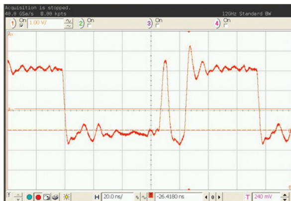
Figure A-27: Example of a clock glitch waveform, a 7.37 MHz clock with a narrow pulse inserted
