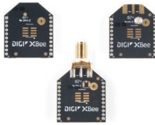
Figure 2-2. XBee module antenna options (courtesy of SparkFun)
