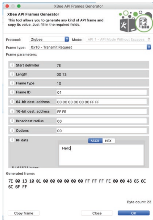
Figure 2-36. Creating the transmit request packet
