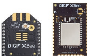
Figure 2-1. XBee 3 form factors
