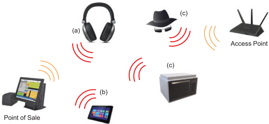
Figure 2-13. Examples of interference affecting the transmission from the Point-of-Sale terminal to the Access Point
