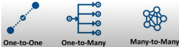
Figure 4-2. Comparison of different Bluetooth network topologies
