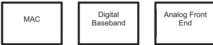
Figure 2-15. The radio includes the MAC and PHY, where the PHY includes the Digital Baseband and the Analog Front End (AFE)
