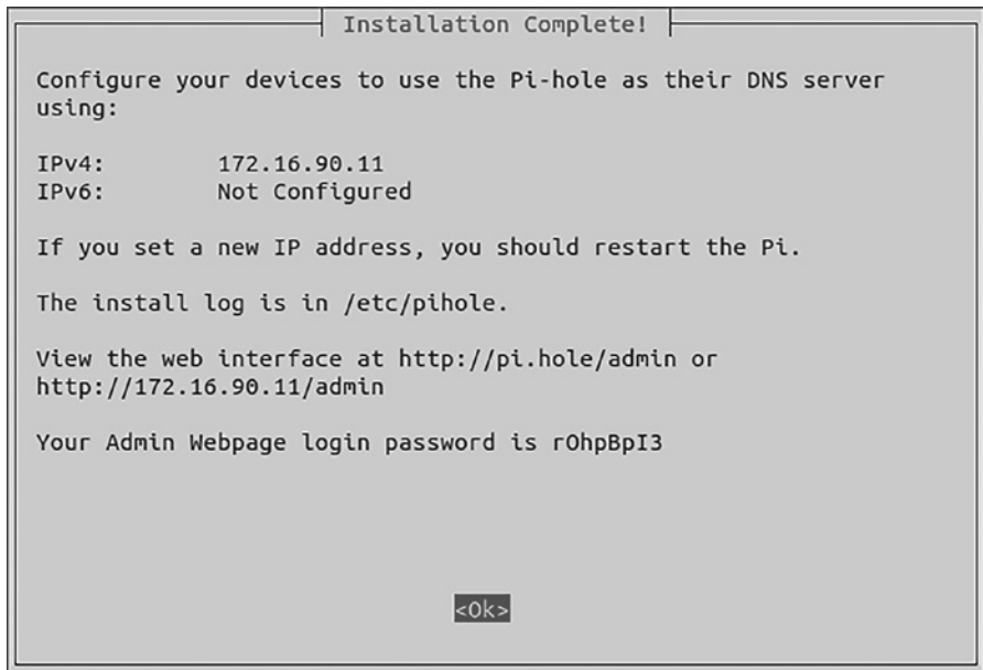
Figure 7-3: Pi-Hole installation complete
