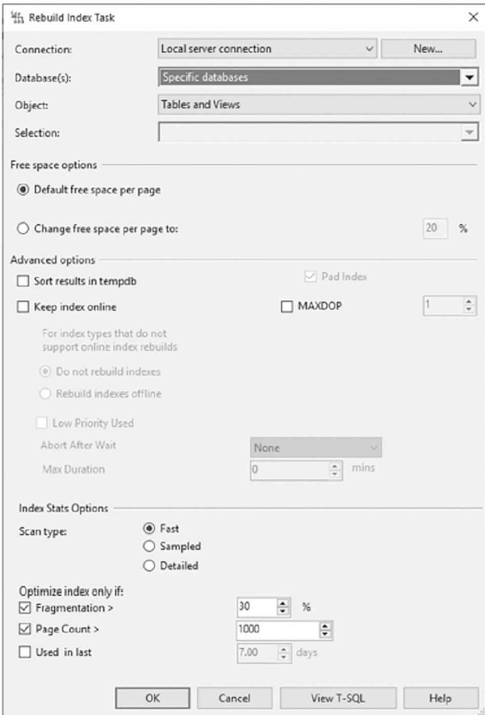
Figure 11-23. Properties window for Rebuild Index Task
