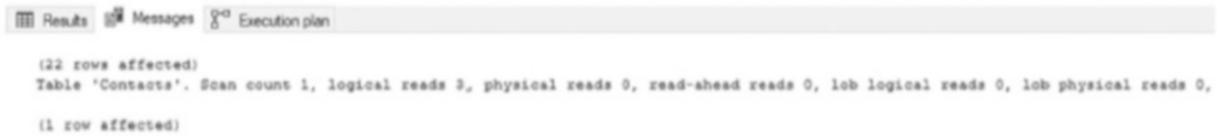
Figure 13-32. Statistics I/O results for the Included Columns pattern with a new index
