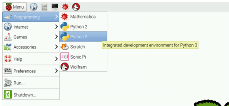
Figure 3.3 Select Menu->Programming->Python 3 to open the Python Shell on your Raspberry Pi.
