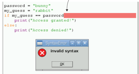
Figure 4.12 A missing colon at the end of an if statement will create a syntax error. Python highlights where the error is located. Add a colon at the end of the line to fix the problem.
