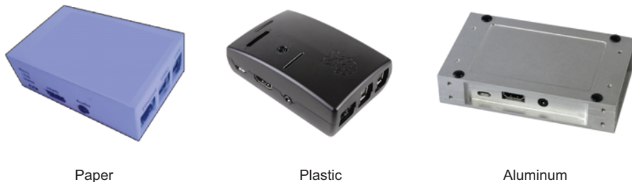
Figure 1.2 A case protects your Raspberry Pi from damage while making it easy to access the ports. Some people use a case to give their Pi a unique personality. You can purchase a case or, better yet, make your own. Plastic cases are the most common, but these pictures show examples of cases made from paper, plastic, and aluminum. You could even try using LEGOs to make one.
