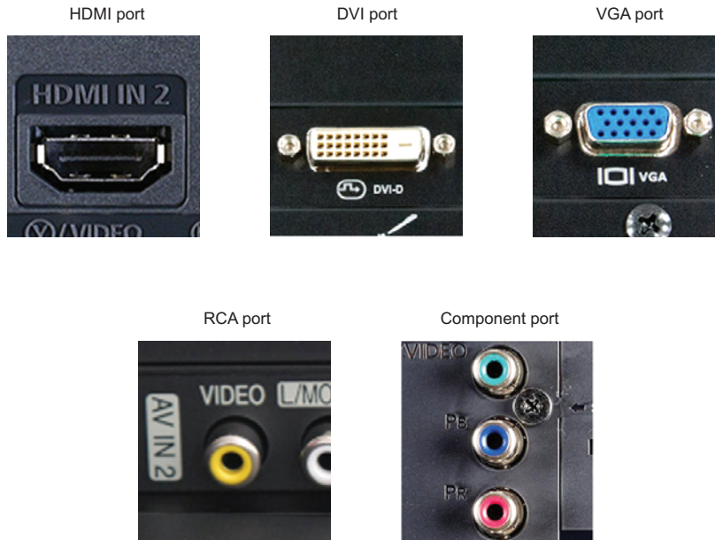
Figure B.8 Common types of video input ports found on TVs and monitors. A Raspberry Pi can connect to any one of these ports. Some ports (DVI, VGA, RCA [or composite], and component) require using special adapters or converters with a Pi.
