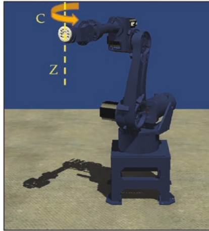
Figure 8-4. A robot in this pose can oppose an infinite torque around the TCP local C axis without performing any actual work
