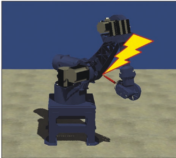
Figure 6-12. Self-collision of the robot with its own body
