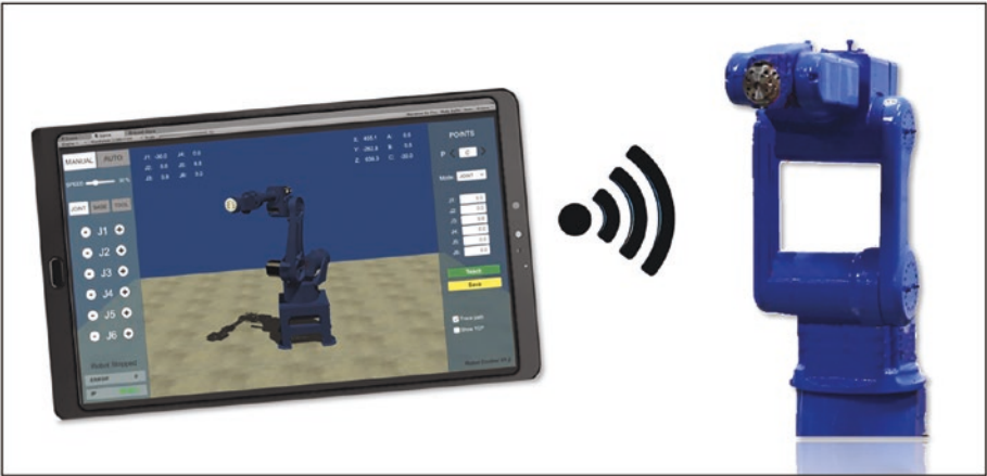
Figure 12-9. Linking the Unity environment to the real robot control system
