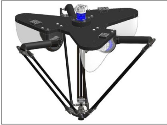
Figure 1-6. A four-axes Delta Robot (with permission from CODIAN)
