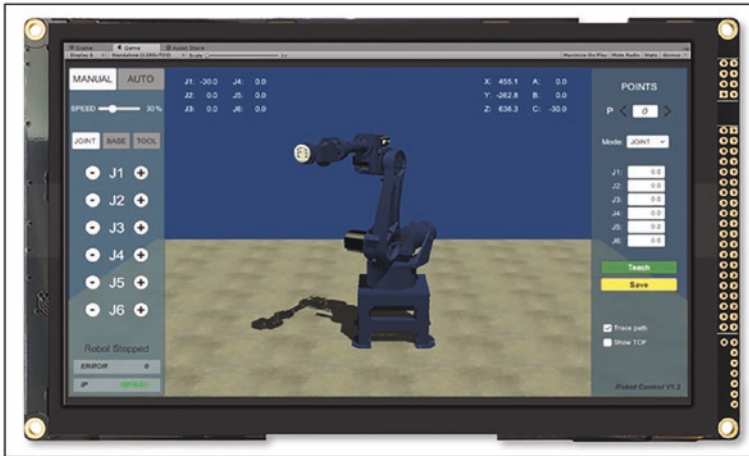
Figure 18-13. A 7-inch TFT display with capacitive touch and SPI interface
