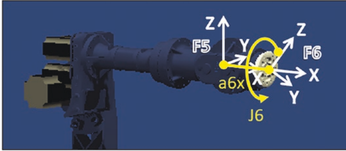
Figure 3-7. FK Step #1: from Frame 6 to Frame 5
