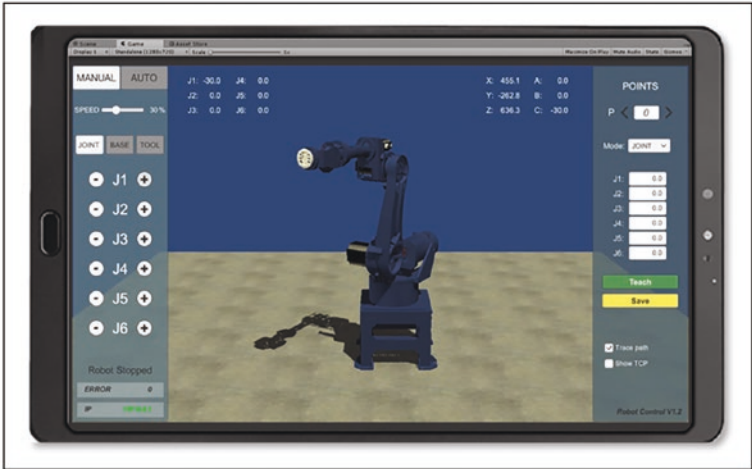
Figure 18-14. A low-cost Android tablet running the HMI for a robot and using a direct Wi-Fi link to the controller
