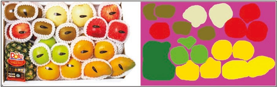
Figure 13-20. Semantic segmentation can be used to identify and measure objects
