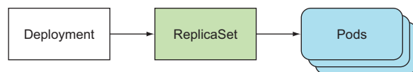
Figure 9.8 A Deployment is backed by a ReplicaSet, which supervises the deployment's pods.
