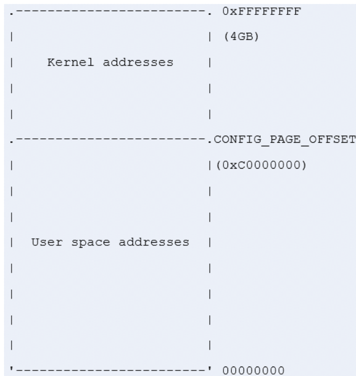
Figure 10.1 – 32-bit system memory splitting
