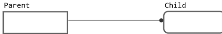
Figure 3-1. One-to-zero or more—a parent row can but does not have to have one or more rows in Child. For child rows to exist, a corresponding parent row must exist
