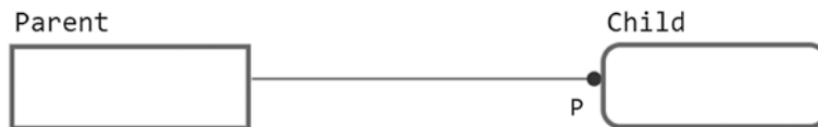
Figure 3-2. One-to-one or more (at least one), indicated by P—for a row to exist in Parent, at least one row must exist in Child and vice versa
