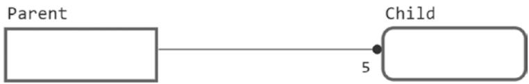
Figure 3-5. One-to-exactly N (in this case, five, meaning each parent must have five children)—for a row to exist in Parent, exactly five rows must exist in Child
