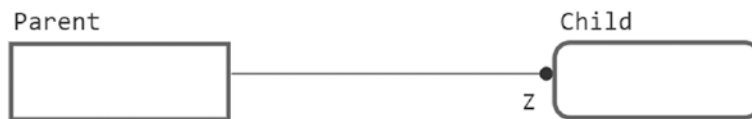
Figure 3-3. One-to-zero or one (no more than one), indicated by Z—a parent row can have one or zero row in Child, but no more. For child rows to exist, a corresponding parent row must exist
