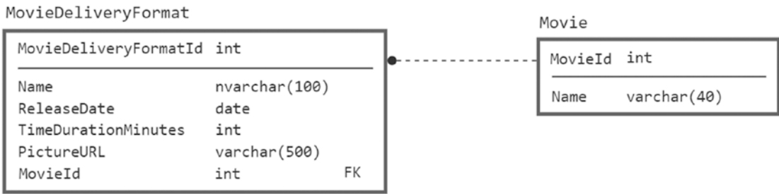
Figure 9-5. MovieDeliveryFormat table with PictureURL datatype set as a path to a file
