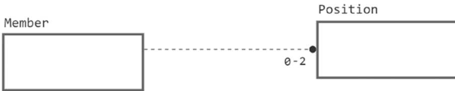
Figure 3-9. A one-to-zero, one-to-one, or one-to-two relationship specifies a maximum limit of two positions per member
