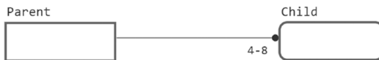
Figure 3-4. One-to-some fixed range (in this case, between four and eight inclusive)—for a row to exist in Parent, between four and eight rows must exist in Child
