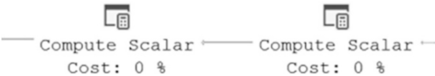
Figure 4-25. Two Compute Scalar operators represent Extra Operators
