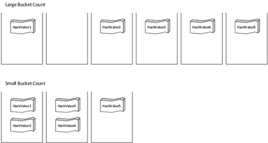
Figure 19-2. Hash values in buckets with a shallow and deep distribution
