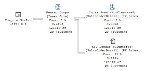
Figure 12.18 – A plan using a FAST N hint
