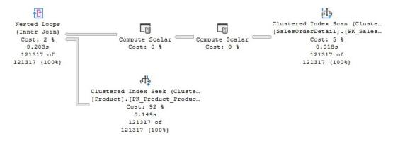
Figure 12.21 – A query using a plan guide
