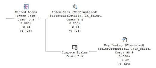
Figure 12.15 – A plan with a Nested Loop Join
