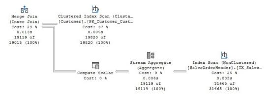
Figure 12.13 – A plan with aggregation before the join
